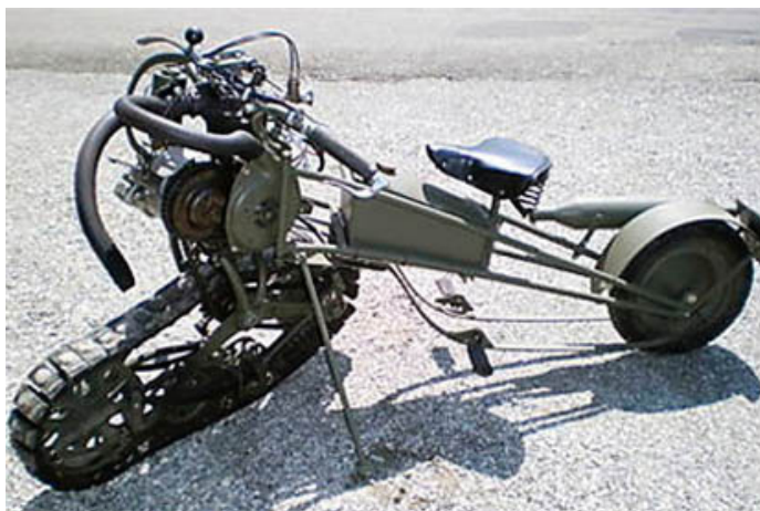
Another front-wheel drive, tracked motorcycle prototype from 1937
