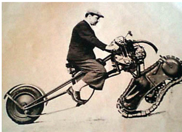
Another front-wheel drive, tracked motorcycle prototype from 1937
