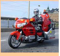
The Retriever's towing rig carries the weight of the car on three wheels so the motorcycle can still be ridden normally. Since the motorcycle is only providing the torque necessary for towing and doesn't have to carry extra weight, the vehicle is easily moved and a six cylinder Goldwing has all of the power you need. The Retriever can tow cars up to 5500 pounds.
